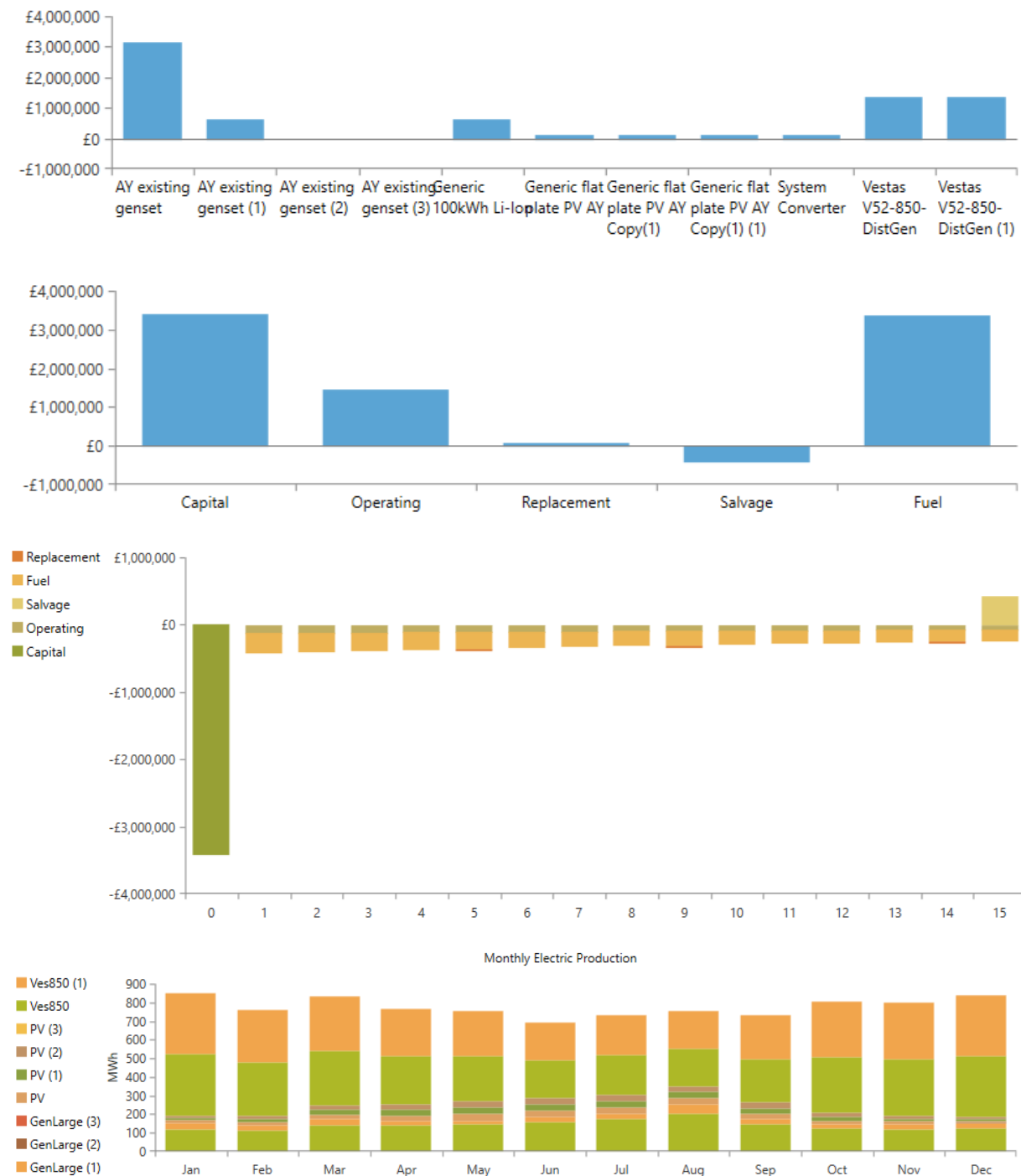
Figure A2. 6 – Key results from the HOMER simulation. Top: Net present cost by system component. Top mid: Net present cost by cost type. Bottom mid: Discounted cash flow. Bottom: monthly electricity production by source.
