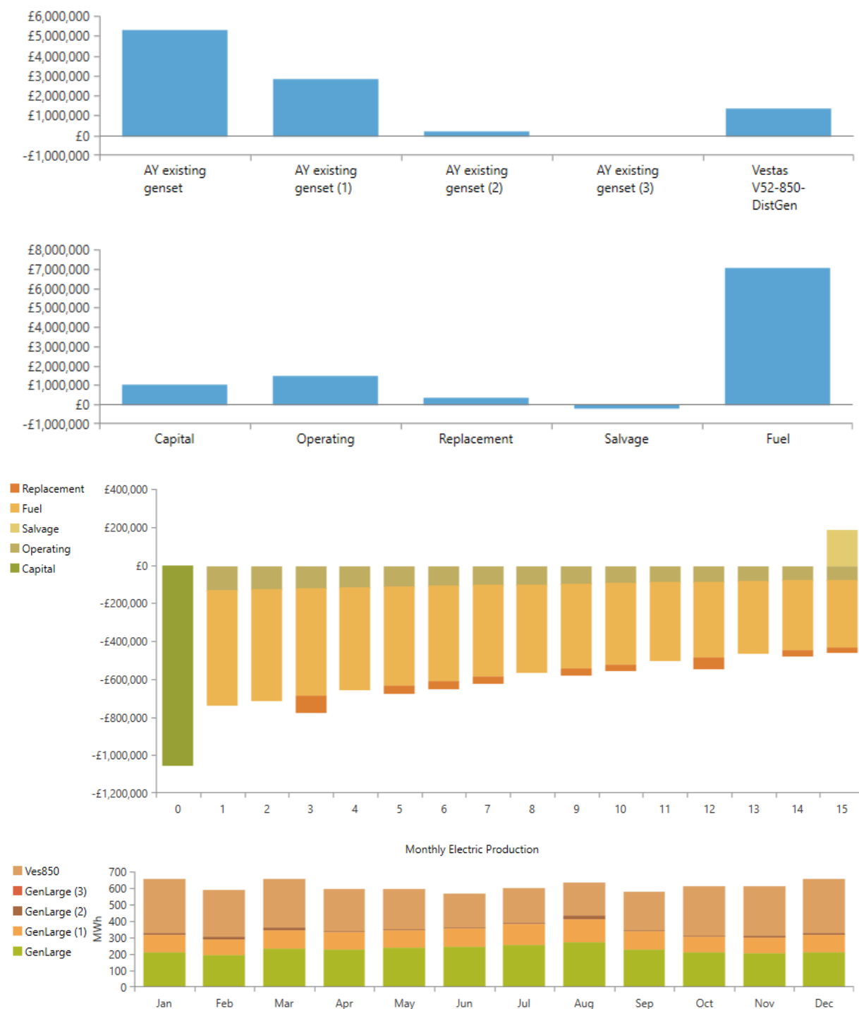
Figure A2. 3 – Key results from the HOMER simulation. Top: Net present cost by system component. Top mid: Net present cost by cost type. Bottom mid: Discounted cash flow. Bottom: monthly electricity production by source.
