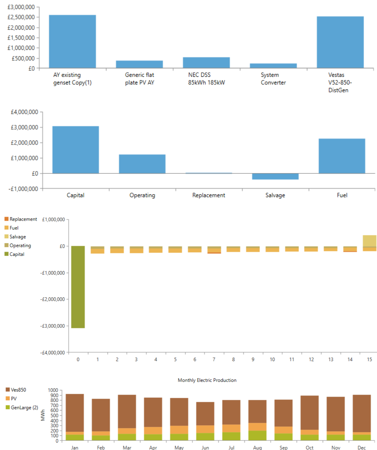
Figure A2. 9 – Key results from the HOMER simulation. Top: Net present cost by system component. Top mid: Net present cost by cost type. Bottom mid: Discounted cash flow. Bottom: monthly electricity production by source.
