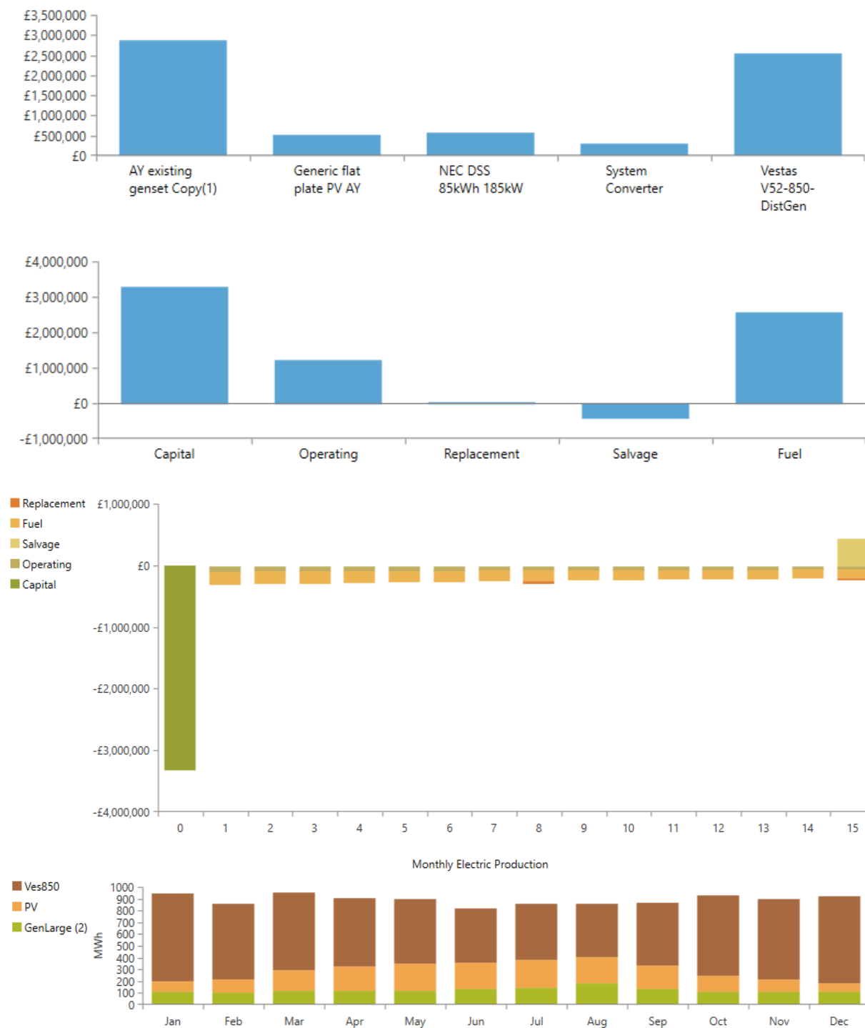
Figure A2.7 – Key results from the HOMER simulation. Top: Net present cost by system component. Top mid: Net present cost by cost type. Bottom mid: Discounted cash flow. Bottom: monthly electricity production by source.
