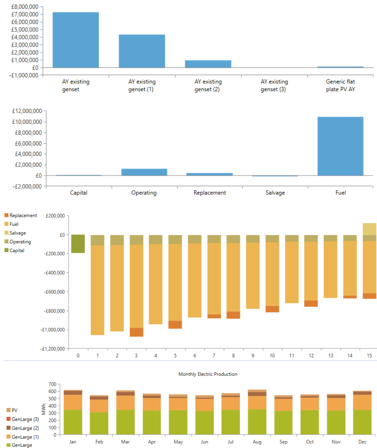
Figure A2. 4 – Key results from the HOMER simulation. Top: Net present cost by system component. Top mid: Net present cost by cost type. Bottom mid: Discounted cash flow. Bottom: monthly electricity production by source.
