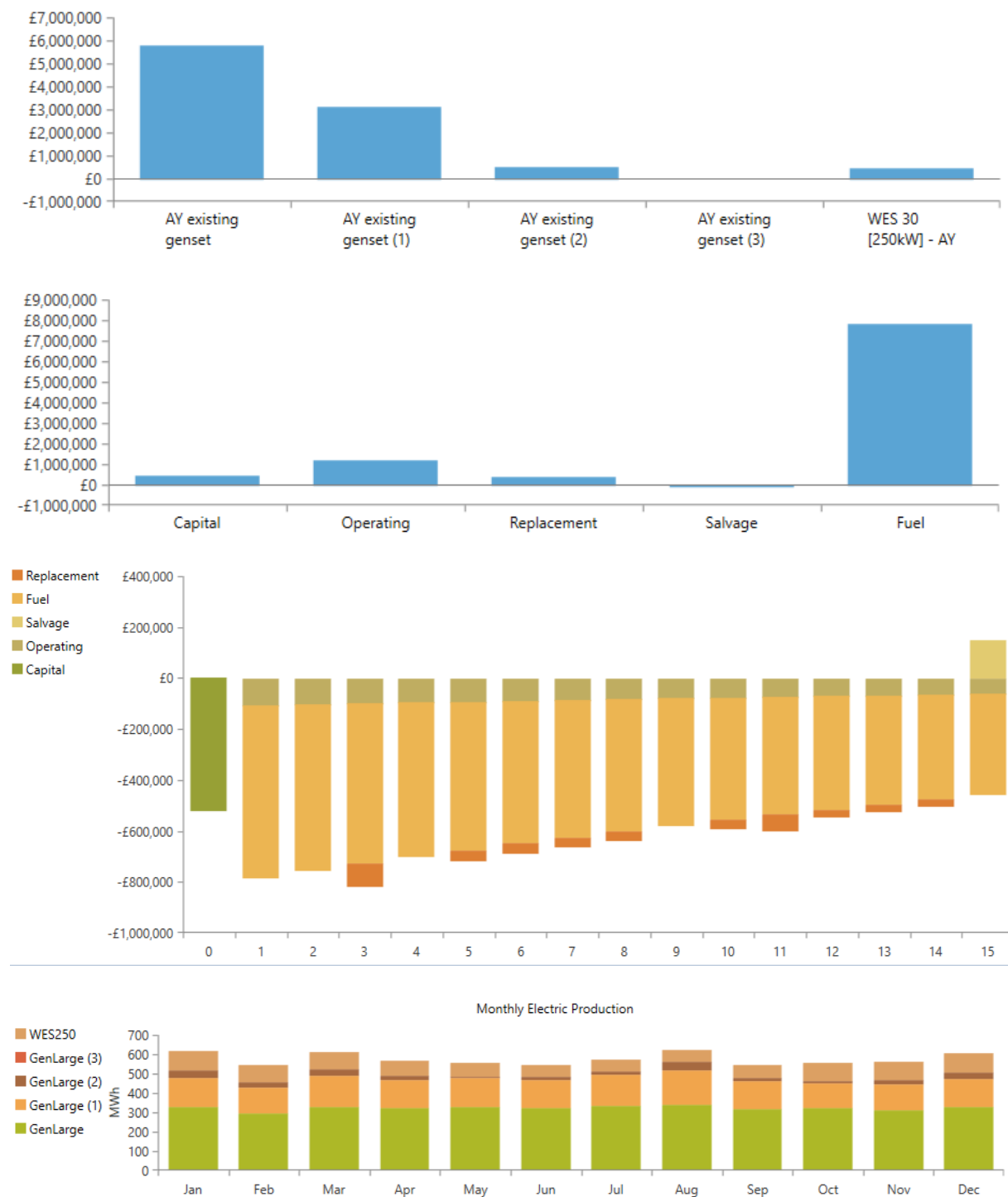
Figure A2. 2 – Key results from the HOMER simulation. Top: Net present cost by system component. Top mid: Net present cost by cost type. Bottom mid: Discounted cash flow. Bottom: monthly electricity production by source.
