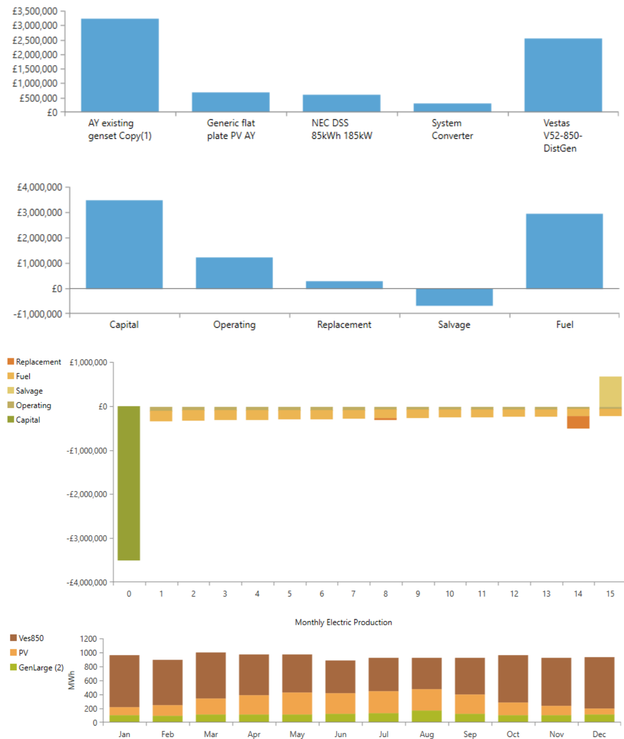
Figure A2. 10 – Key results from the HOMER simulation. Top: Net present cost by system component. Top mid: Net present cost by cost type. Bottom mid: Discounted cash flow. Bottom: monthly electricity production by source.
