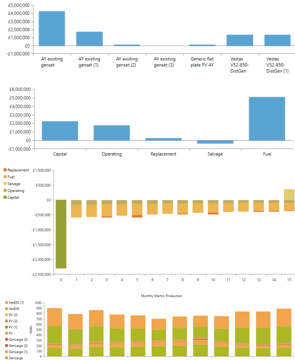
Figure A2.5 – Key results from the HOMER simulation. Top: Net present cost by system component. Top mid: Net present cost by cost type. Bottom mid: Discounted cash flow. Bottom: monthly electricity production by source.
