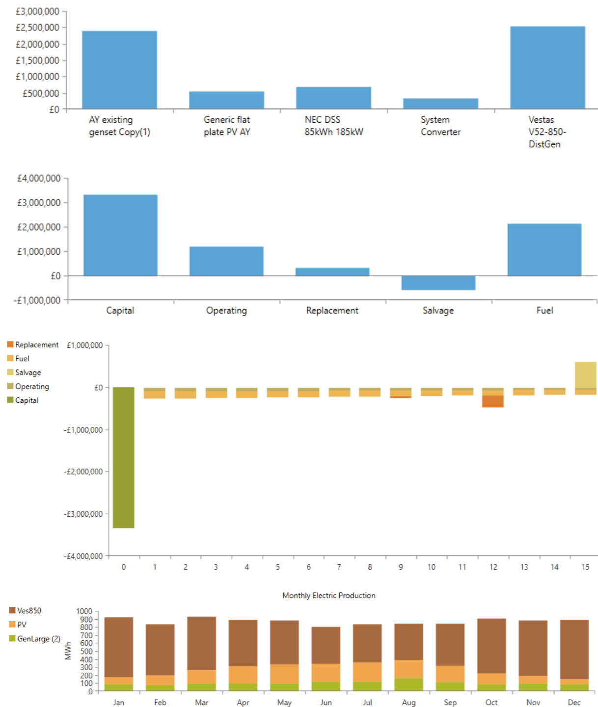
Figure A2. 8 – Key results from the HOMER simulation. Top: Net present cost by system component. Top mid: Net present cost by cost type. Bottom mid: Discounted cash flow. Bottom: monthly electricity production by source.
