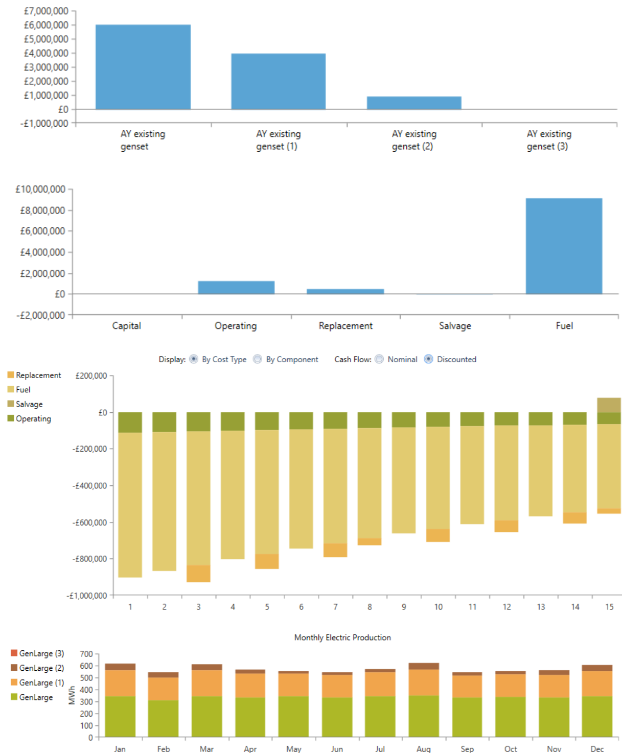
Figure A2. 1 – Key results from the HOMER simulation. Top: Net present cost by system component. Top mid: Net present cost by cost type. Bottom mid: Discounted cash flow. Bottom: monthly electricity production by source.
